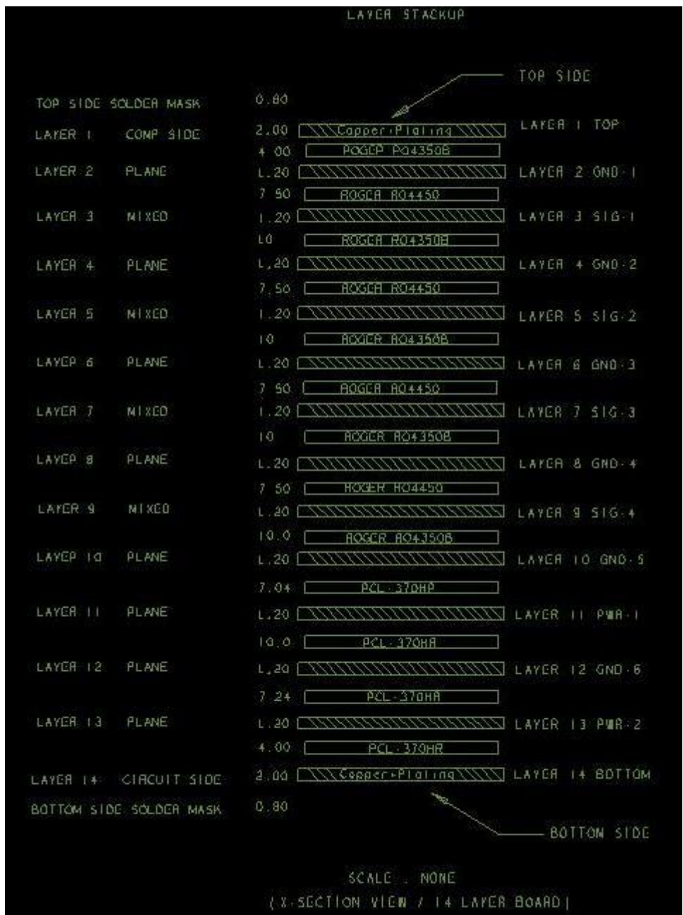
Figure 2: Stackup with Rogers dielectric for high-speed signal layers
